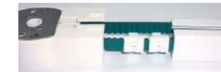
2.Install the second belt holder beside the first belt holder (one tooth space, on the left side), as above photo shown.
