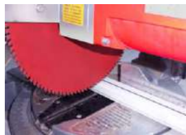
Cut and prepare rail PS: Please use professional cutting machine
