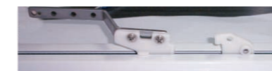
4.Slide the sub carrier to master carrier, connect the master carrier and sub carrier.
